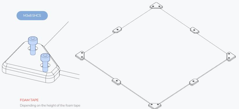
between the panels and the frame, you will likely have to use larger sized clips depending on it's thickness.
