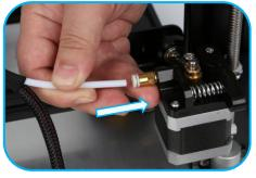
Insert the Teflon pipe into the quick connector
