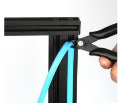
Cut off the excess material with the diagonal pliers
