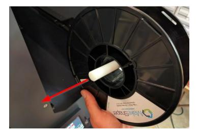
Orient the spool so the filament pays off the front side (or underneath) of the spool.
