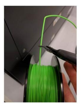
Cut the end of the new spool square as well. Align the ends and press forward as it feeds into the extruder
