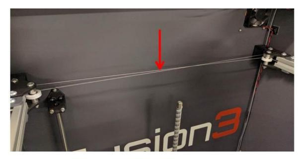
Use a light finger touch on the cables to ensure they are not slack. A wide range of tension is acceptable; as long as the cables are not actually loose they are fine.
