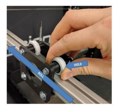
If there is little to no resistance, the preload is too loose. Use the preload adjustment wrench (download from our website: <a href="https://fusion3design.com/manuals">https://fusion3design.com/manuals</a>) to rotate the eccentric cams to adjust the preload. You can also use two 13mm wrenches with the handles lined up.
