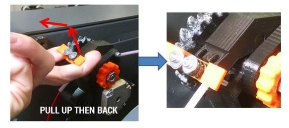
Pull up and back (towards yourself) to disengage the springs from the idler bar.
