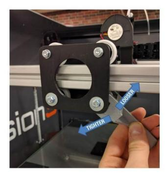
NOTE: It's possible to over-tighten the cams. Aim for roughly 10 in-lb of resistance when you slide the carriage while holding the wheel still.
