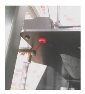
Turning it **counter-clockwise** will **lower** the bed corner. And turning it **clockwise** will **raise** the bed corner.
