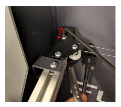
Once you adjust the pulley, tighten the screw and re-check the square.
