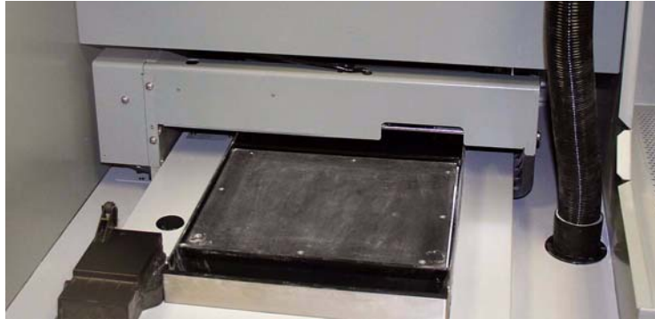
A clean, properly prepared Build Bed
