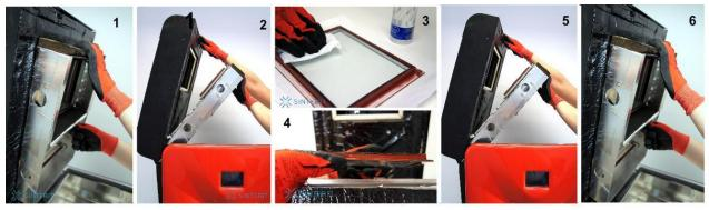
Photo 28. Replacement of the glass protecting laser
