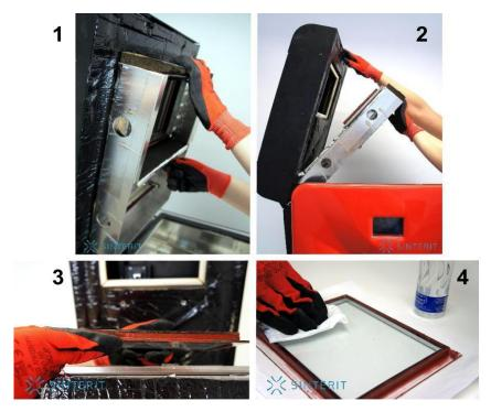
Photo. 24. Cleaning the protective glass laser
