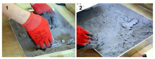
Photo 26. The method of crushing the remnants of print and pre-sieving
