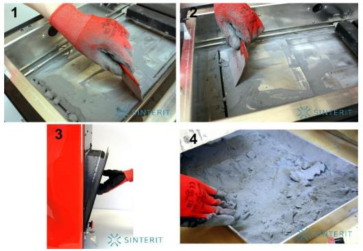
Photo 23. Removing the remaining powder from inside
