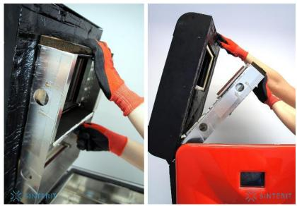
Photo 9. Correct holding unit heaters while loosening
