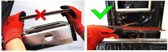
Photo 10. Incorrect and correct positioning of the protective glass laser module heaters.
