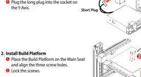
Note: (1) The device is pre-leveled in factory. There is no need to level the ound place. (3) (2) It is only need to install three screws. Do not remove the top right screws.
