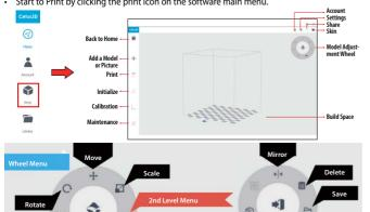
**Note:** Initialization is required every time when the machine is powered on, this is in order to determine the correct position.
